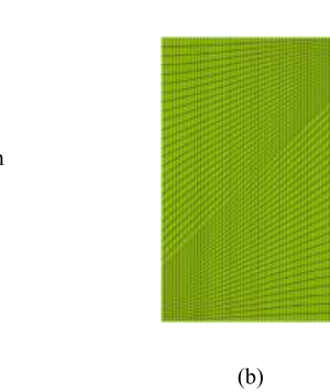
Fig. 8. Consolidation of a block with inclined discontinuity (a) Geometry and boundary conditions (Adapted from Lamb et al. (2013)), (b) Finite element mesh used in the DFM.
